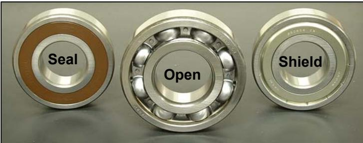
The capacity of a bearing will be the same regardless if it has seals, open, or shielded. All three bearings will accept the same load and produce the same life. The three bearing will have different speed limits. Speed limits are determined by how hot
