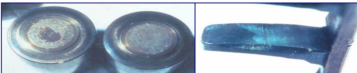
**Rusting, Corrosion :** Rusting and corrosion is oxidation of the steel. Can cause pits on the surface of the rings & rolling elements
