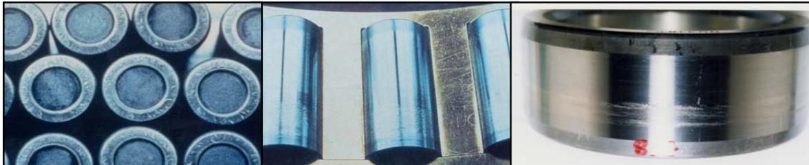
**Excessive Wear** : Surface deterioration due to heavy sliding friction between the contact areas of the bearing components
