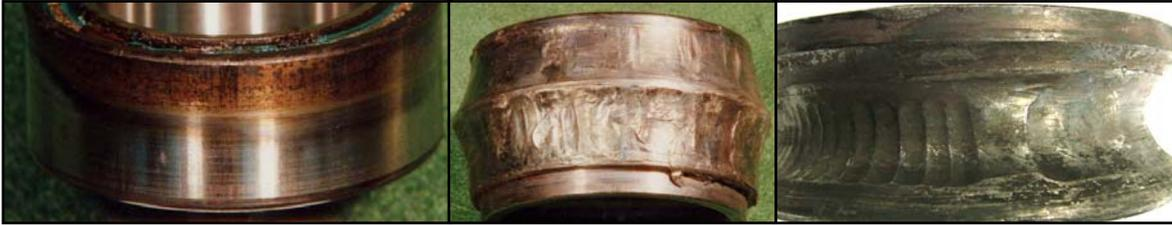
**Flaking:** Repetitive Heavy stress cycle between the bearing raceways and rolling elements resulting in surface fatigue cracks and spalls
