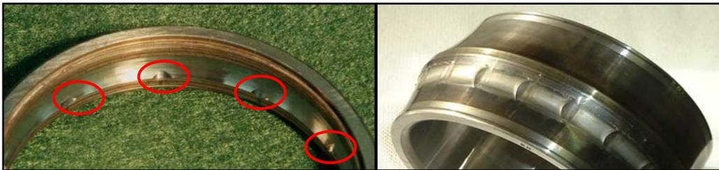
**False Brinelling:** The occurrence of elliptical wear at ball or roller spacing due to an excessive external vibration
