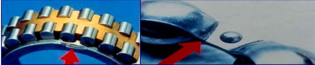
**True Brinelling:** The occurrence of dents on the raceways that are the result of exceeding the elastic limit of the steel.
