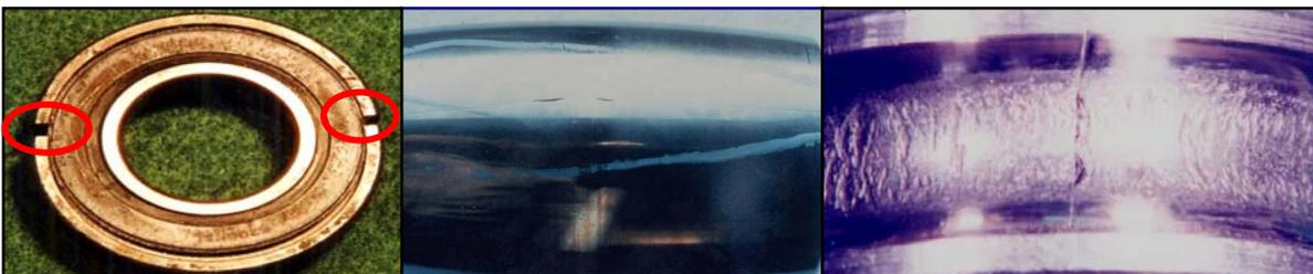
**Fracture:** Cracked inner ring rib. Broken retainer.
